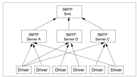
Figure 6-8 Three-way SMTP cluster using round-robin DNS
