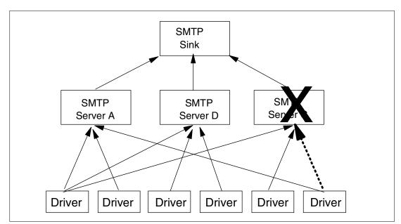
Figure 6-9 Round-robin DNS with one failed host
