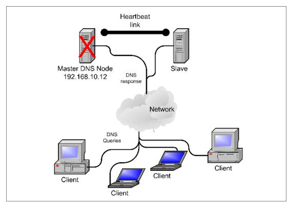
Figure 4-2 Failed master DNS server
