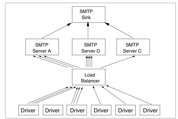
Figure 6-10 Using a load-balancer
